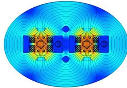
Figure 1: 4.5 Tesla C-dipole for an ultimate-energy hadron collider. Each beam tube has a side SR channel.
