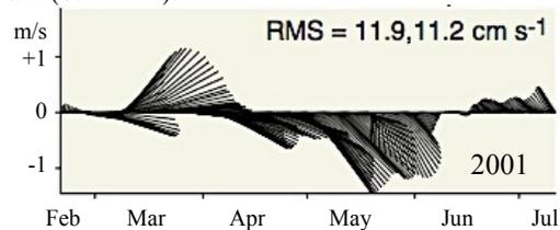
Figure 4: Velocity field history of currents at 122 m depth at an example site in Gulf of Mexico.
