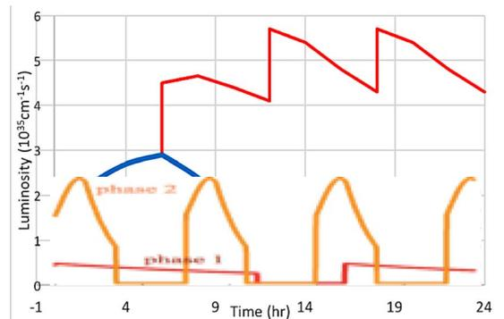
Figure 8: Instantaneous luminosity for a single filling of protons beam (blue), and for top-up stacking every 6 hours (red), and for FCC-hh in orange [10].
