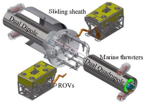
Figure 6: Demountable joint connecting half-cells of the pipeline cryostat. Shown are the valve trees for each umbilical, the retractable sheath, the marine thrusters, and two ROVs assembling joints.
