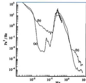
Figure 5: Power spectra of pressure fluctuations near the sea floor, for a) 5 cm/s and b) 30 cm/s currents.
