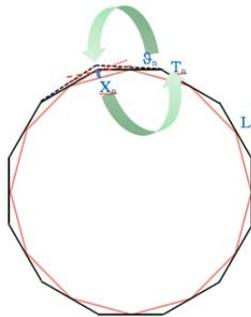
Figure 7: Schematic of detection of a local displacement  $\vartheta_n$  of single quadrupole and correction using trim dipole  $T_n$ .
