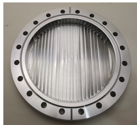
The vacuum vessel for the zero-length ICF 203 NEG pump
