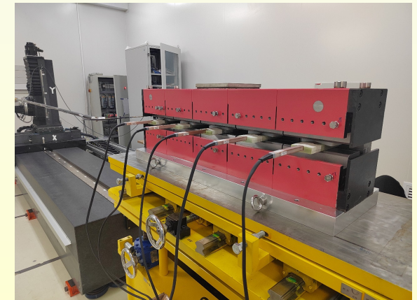
HEPS dipole in test
