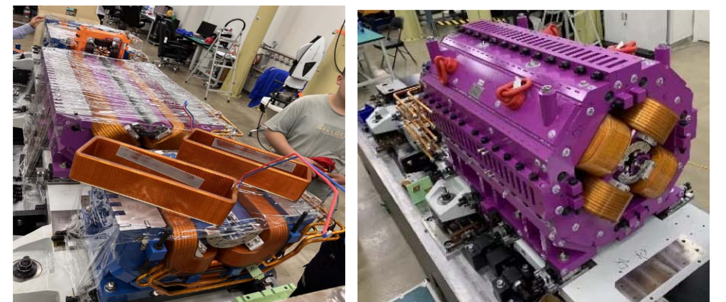
Installation of the sextupole & Mover
