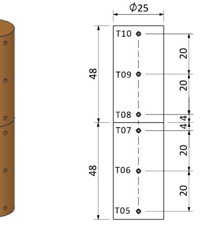
The temperature distribution along the length of the specimens is observed to follow a linear dependence with a drop at the interface ( $\Delta$ T). By knowing heat flow across it (Q) and the interface area (A), the thermal contact
