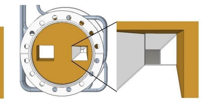
Fully opened slits Yaw =  $-1^{\circ}$ , Pitch =  $-1^{\circ}$
