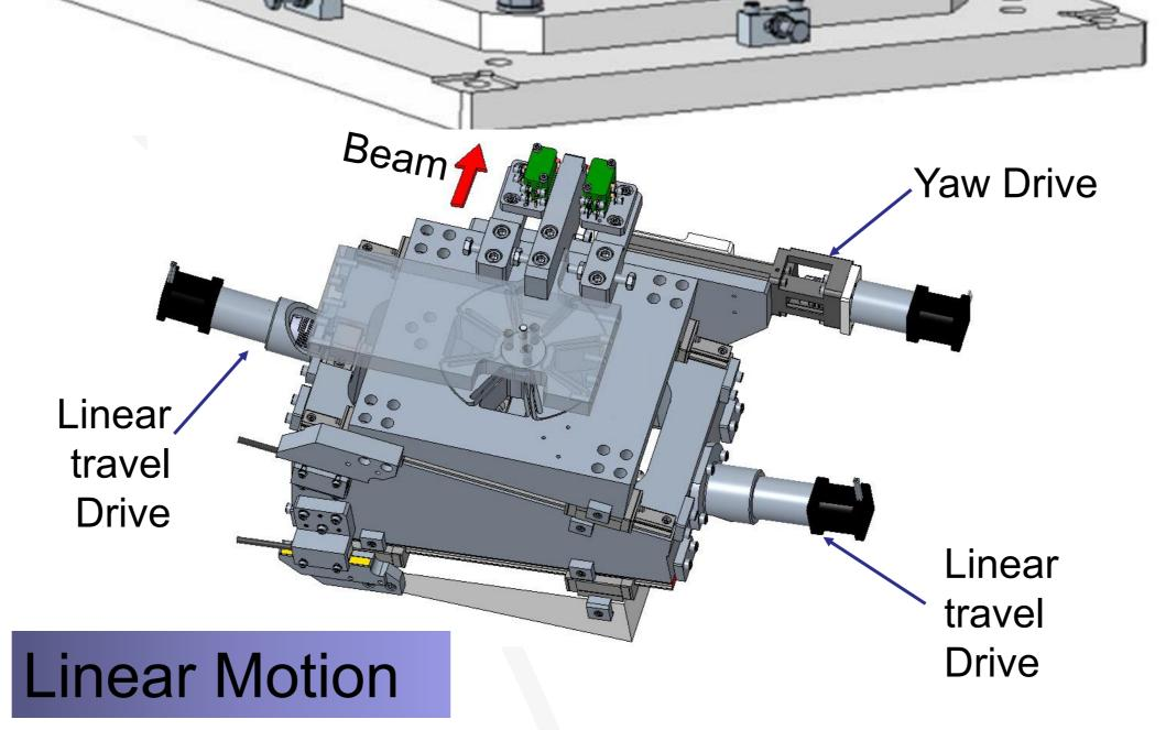
A compound motion is needed to produce a purely horizontal or vertical motion. The scan distance is +/-4.5 mm at motion hard stops.
