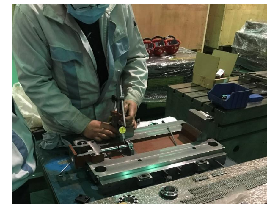
Figure 9. Installing test of ball screw.
