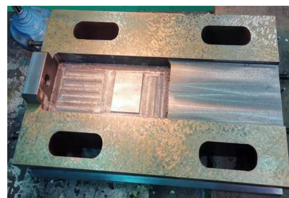
Figure 8. Surface after scraping and grinding.
