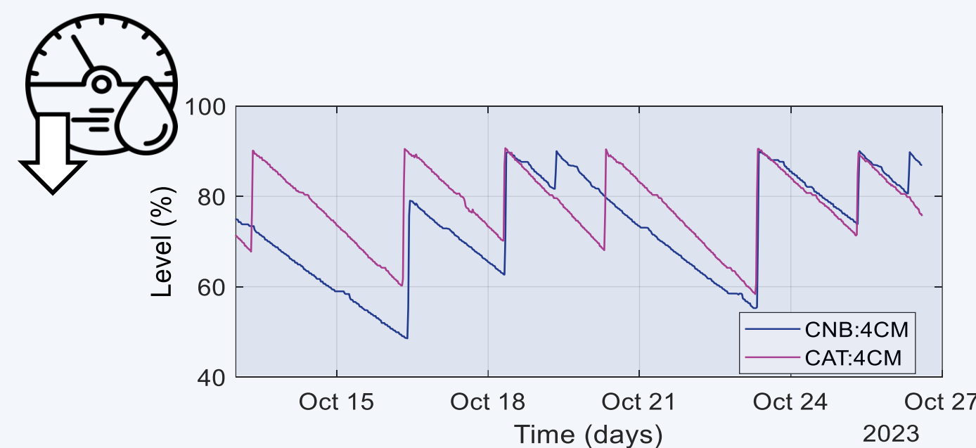
The maximum level of the LN2 vessels is limited to 90% to prevent ice formation near the needle valve.
