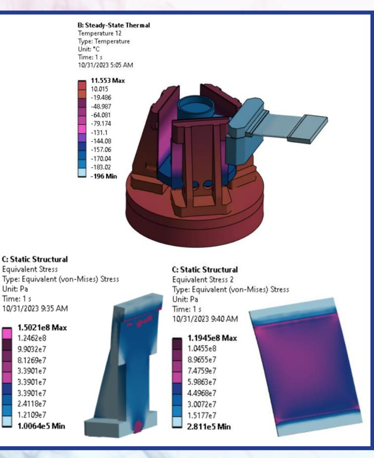
The design of optical elements compasses different development areas, such as optics, structures, dynamics, thermal, and control. Thermal designs of mirrors aim to minimize deformations, whose usual requirements are around 5 nm RMS and slope errors in the order of 150 nrad RMS.
