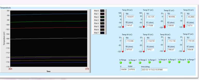
LabView interface to temperature acquisition and heaters control.
