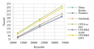
Comparison of Nusselt calculated by CFD to experimental correlations for channel 10 mm diameter.
