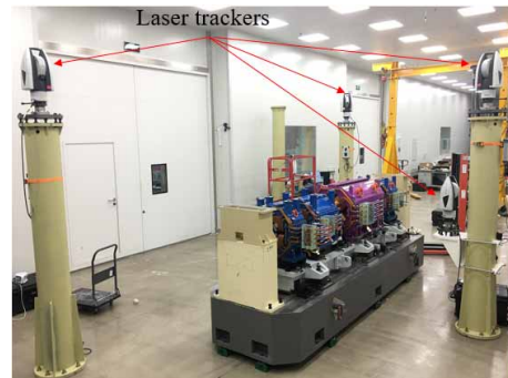
Figure 2: Laser tracking interferometer system.
