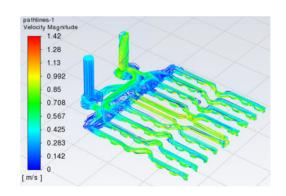
Figure 6: CFD simulation of detector cooling component using ANSYS Fluent.
