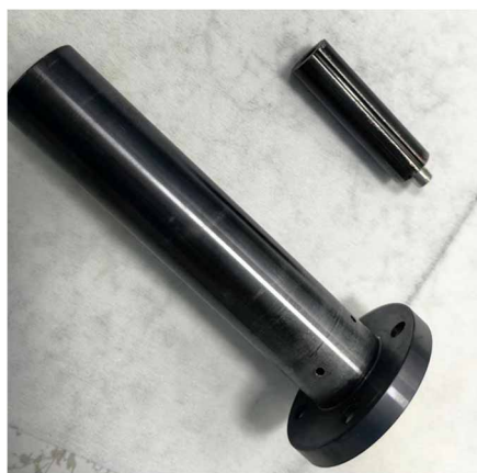
Figure 3: Sleeve system with MoS 2 coating.
