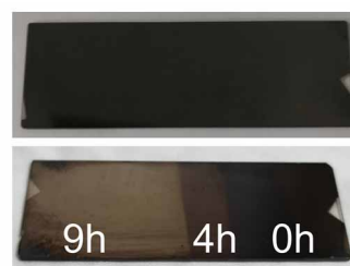
Figure 9: Cleaning of Al-coated mirror with Ar/H 2 .
