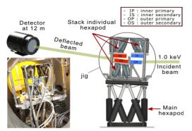
Figure 2: Mirror Module JIG and reflection scheme (from PTB).
