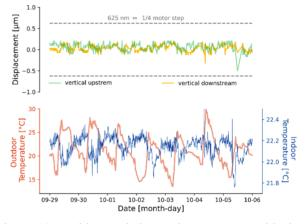
Figure 10: Position variation and temperature with time (fine close loop tunning).
