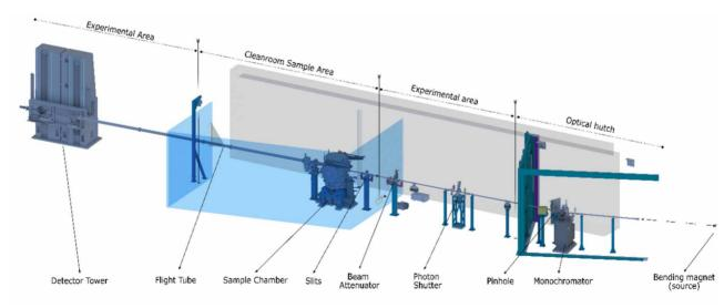
Figure 3: MINERVA layout presenting the main components of the beamline.
