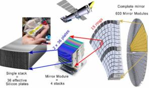
Figure 1: ATHENA Telescope Multiscale Optics Scheme
