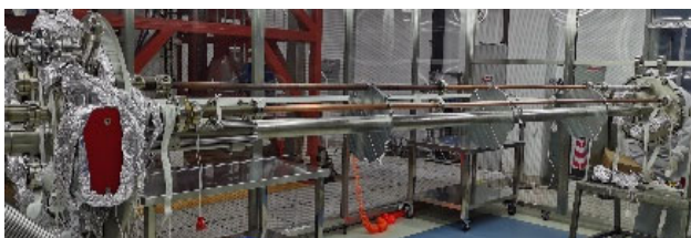
Figure 2: (a) Massive produce facilities of NEG coating, (b) Vacuum chambers were installed in parallel and series to massive coating.
