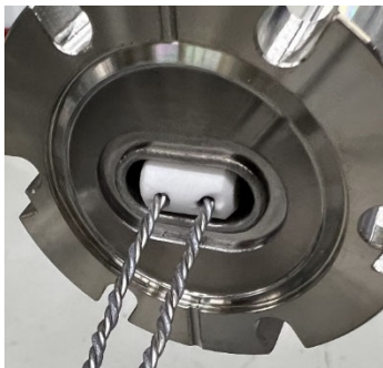
Figure 7: Prototype of racetrack shape vacuum chamber, two cathodes were mounted along the axis direction.
