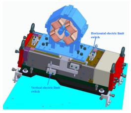
Figure 2: Limit switches in quadrupole support.
