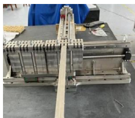
Figure 8: Prototype of stripper foil motion mechanism.
