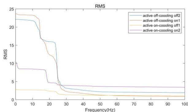
Figure 15: Pitch vibration comparison between mirror and granite with and without cooling when active vibration isolation system on and off in statistics.
