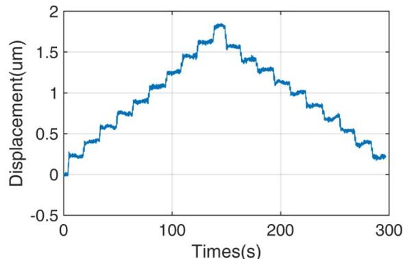
Figure 8: X translation was tested with each step of 167 nm when airpads were pressurized.
