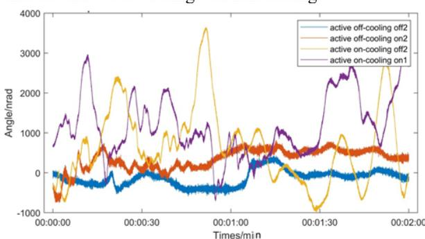
Figure 17: Waveform of pitch angle comparison between mirror and ground with and without cooling when active vibration isolation system on and off.
