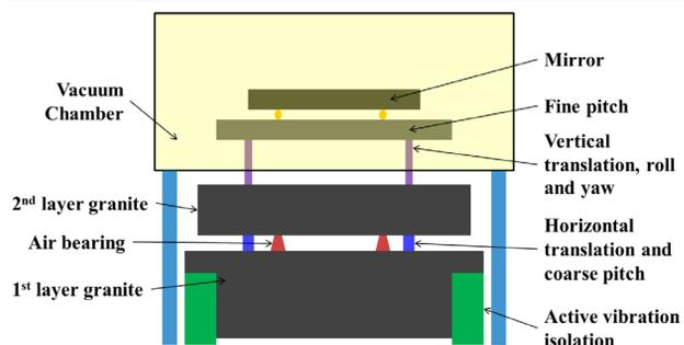
Figure 2: Schematic of the mirror chamber system.
