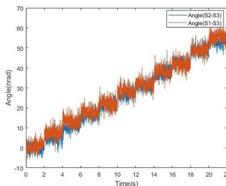
Figure 11: Fine pitch was tested with each step of 2 nm by the piezo, resulting about a 5 nrad resolution.
