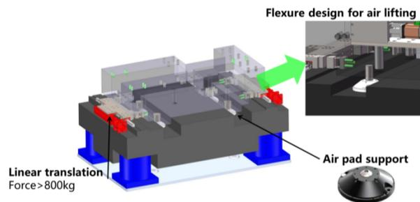
Figure 4: Model of coarse pitch and X-translation with air pad support.
