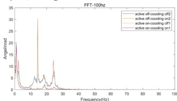
Figure 12: Absolute pitch vibration comparison with and without cooling when active vibration isolation system on and off in spectrum.
