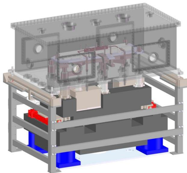
Figure 3: 3D model of the mirror chamber system.
