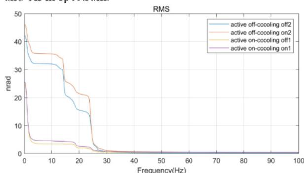
Figure 13: Absolute pitch vibration comparison with and without cooling when active vibration isolation system on and off in statistics.
