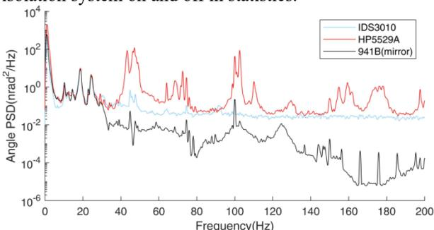
Figure 16: Spectrum comparison of pitch angle with different measurements when active vibration isolation was enabled and water cooling was functioning.
