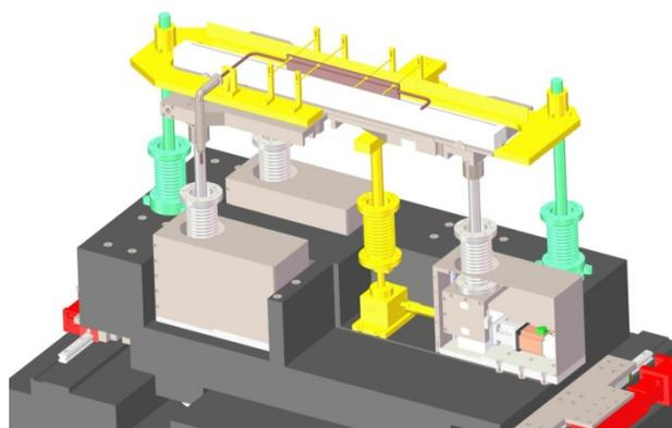
Figure 5: Mirror cooling was decoupled to the cooling blade, while the movement of the water cooling was coupled to the vertical translation of the mirror.
