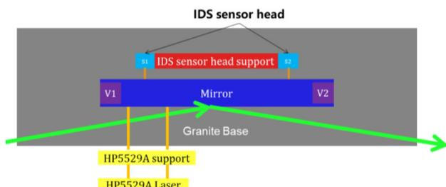
Figure 7: Measurement set up for pitch angle of the mirror.
