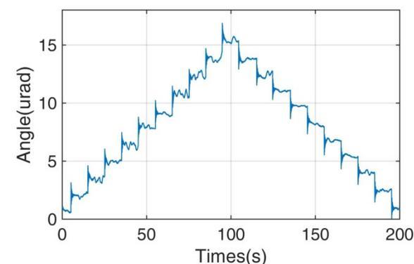
Figure 9: Coarse pitch was tested with each step of 1.5 μrad when airpads were pressurized.
