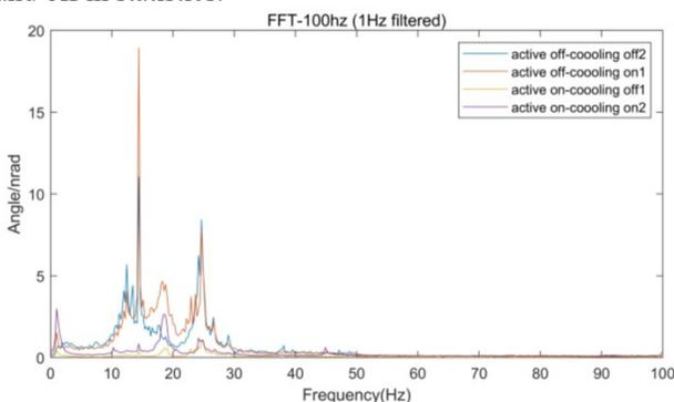
Figure 14: Pitch vibration comparison between mirror and granite with and without cooling when active vibration isolation system on and off in spectrum.
