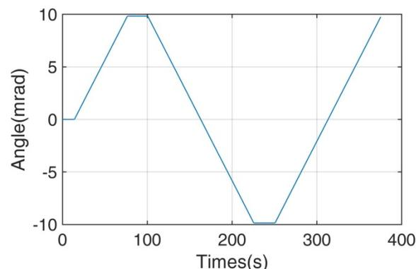
Figure 10: Coarse pitch range was moved from -10 mrad to 10 mrad.
