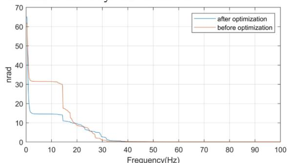
Figure 18: Comparison of stabilities with the optimization of the joints connecting to the pillars of the gearboxes.
