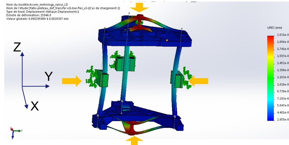
Thermal drift of xtal cage should not induce a metrology frame deformation above the specifications for a short scan range (1 deg), i.e a short term drift.
