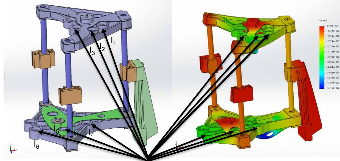
change of static error X1/X2 due to gravity / deg
