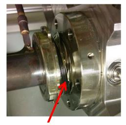
Damage of bellows during manipulation
