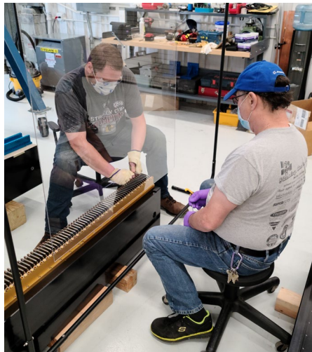
ID Technicians Removing Magnets from Magnetic Structure with Covid Controls in Place
