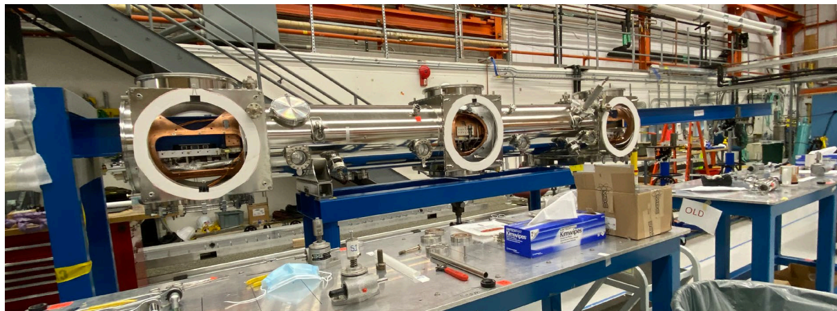
Vacuum vessel being moved over the cold mass assembly
