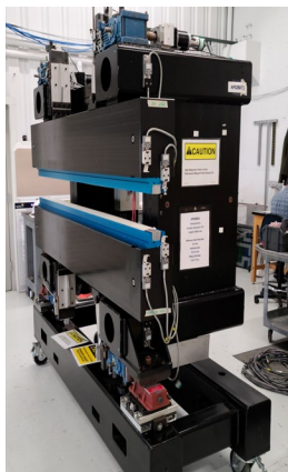
Magnetic Structures Assembled onto Spare GSM
