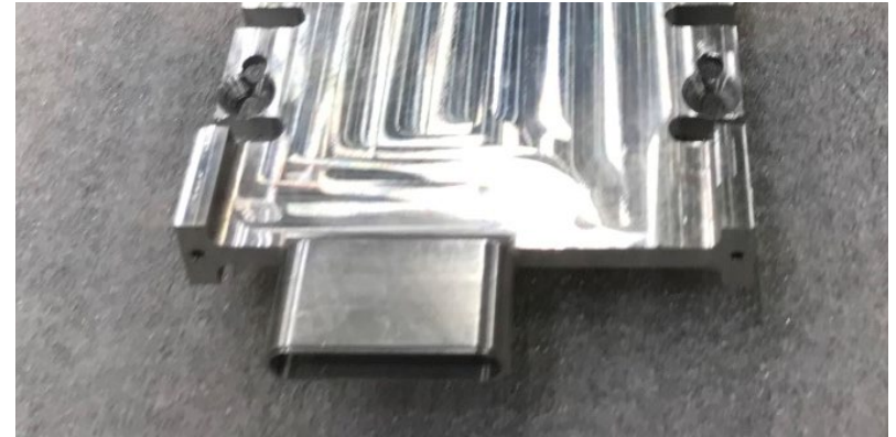
SCU VC Post Machining (Center Region is 7.1 mm tall for reference)
