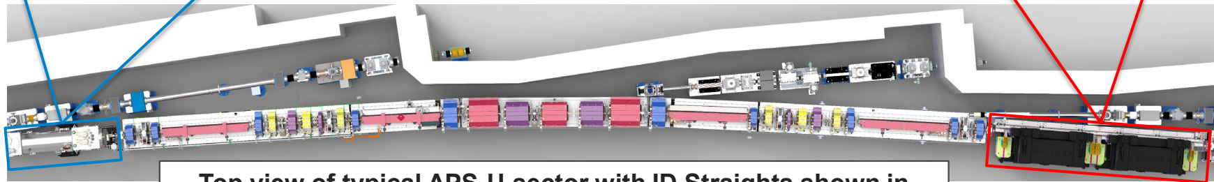
Top view of typical APS-U sector with ID Straights shown in blue (SCUs) and red (HPMUs)
