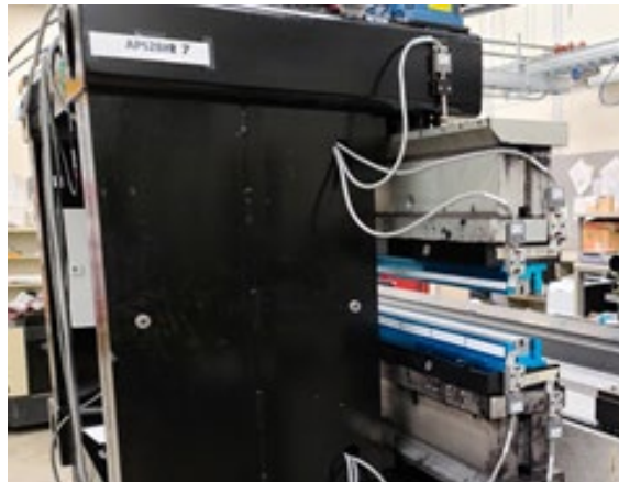
New 2.8 cm Period Device with Monokeeper
