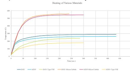
Figure 6: Heating Curves for Various Materials and Coatings
