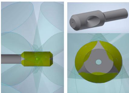
Figure 3: Redesigned sample tube holder (a) looking downstream, (b) end view with heat flux pattern in yellow, and (c) view looking upstream with  $\pm 45^\circ$  exit opening to collect diffraction data
