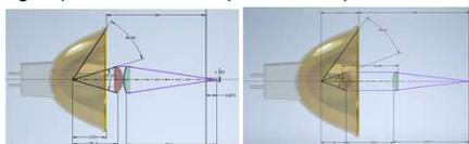
Figure 2: IR lenses with focus (a) behind sample and (b) at sample center
