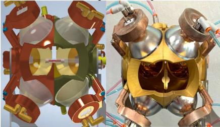
Figure 1: XPD Infrared Sample Furnace looking upstream (a) rendering (b) photo
