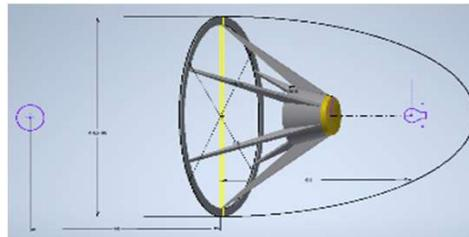
Figure 5: Design of a secondary spherical reflector to capture forward-directed IR rays
