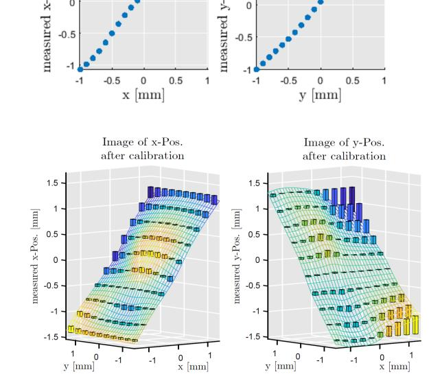
Position after calibration; bar/color: difference between measurement and calibration In an area of 1x1mm<sup>2</sup>: Calibration-Accurancy: 0.15mm, Sensitivity to position changes in all area
