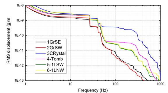
Figure 9 Integrated RMS displacement
