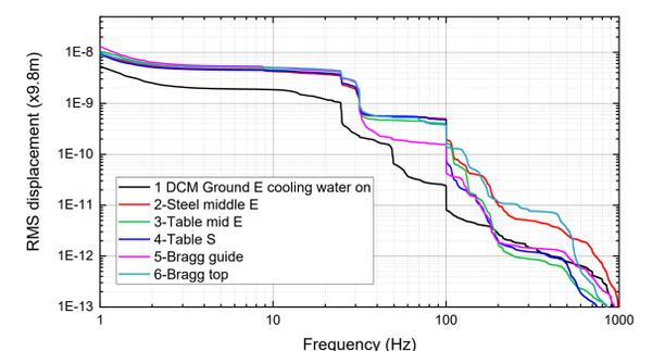
Figure 11 Integrated RMS vibration
