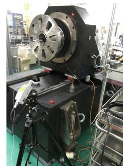
Figure 8 Horizontal direct drive spindle
