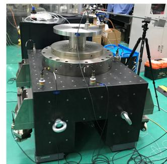
Figure 6 Vertical direct drive spindle
