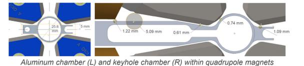
Aluminum chamber (L) and keyhole chamber (R) within quadrupole magnets
