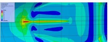
Von-Mises stress results of the Al inline absorber thermal-structural FEA (max stress 46.3 MPa)
