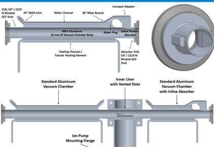
Cross-sectional overview of a standard aluminum chamber with inline absorber (top left), bimetal flange showing the inline photon absorber (top right), cross-sectional overview of an aluminum pumping cross (bottom)
