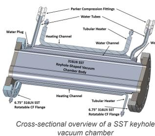
Cross-sectional overview of a SST keyhole vacuum chamber
