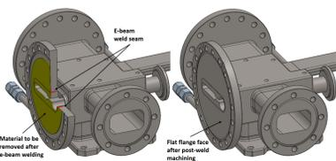
Explanation of the flange e-beam weld for the A:VC6 cross and the keyhole chambers (not shown)
