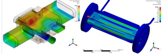
Temperature results from A:VC6 cross bakeout analysis (max 188°C, min 172°C)
