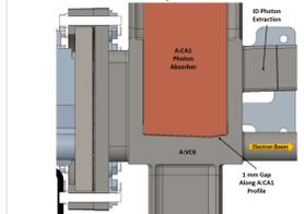
Top cross-sectional view of the discrete photon crotch absorber within the A:VC6 cross body
