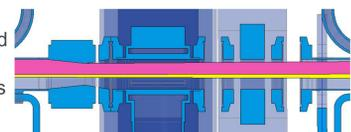
Top cross-sectional view of the ray trace through a copper chamber, cross, and BPM demonstrating shadowing from an inline absorber
