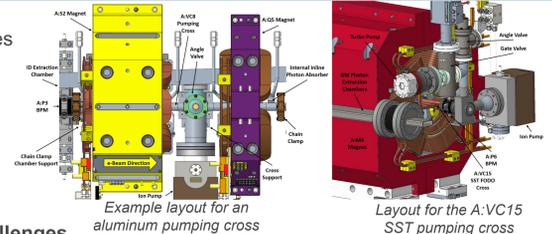
Example layout for an aluminum pumping cross
