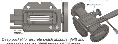
Deep pocket for discrete crotch absorber (left) and serpentine cooling (right) for the A:VC6 cross
