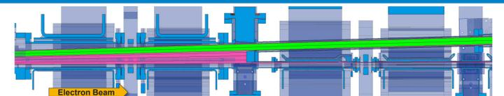
Top cross-sectional view of the ray trace through keyhole chambers, BPM, cross+crotch absorber, aluminum chambers, and photon extraction chambers
