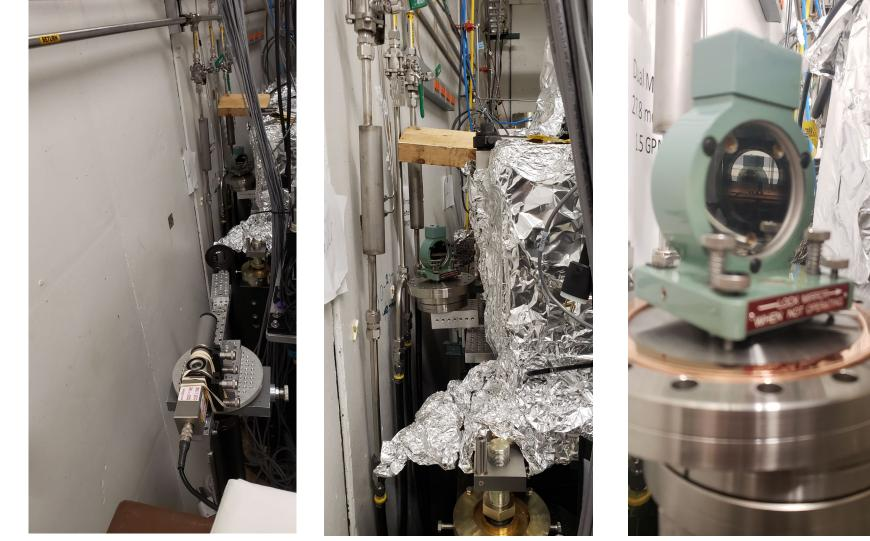
*In situ* autocollimator readings of both mirrors have been made under normal operating conditions utilizing viewports and a VLM in the case of downstream/outboard mirror which is inward facing.
