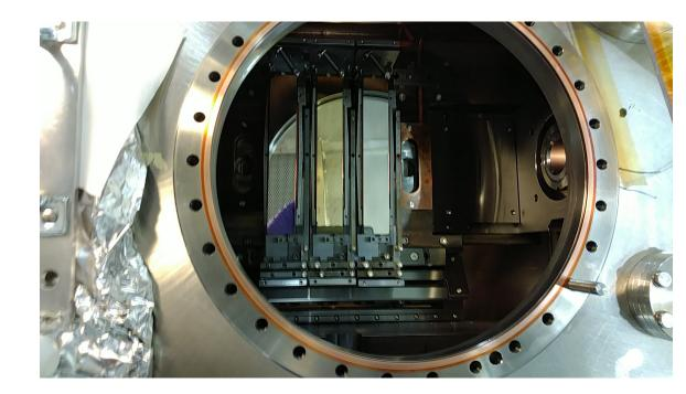
View thru open access port on 4-ID-C SGM showing third grating installed. Photo on bottom right shows how autocollimator was used to set new grating to have same pitch and roll s existing gratings.
