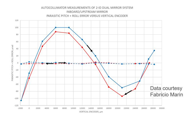
4-ID-XTIP M5 MIRROR TESTING PITCH ANGLE MEASURED AT A POINT ON MIRROR LOCATED ~2 INCH UPSTREAM OF POLE MEASUREMENTS MADE WITH CONEX-I DS AUTOCOLLIMATOR
