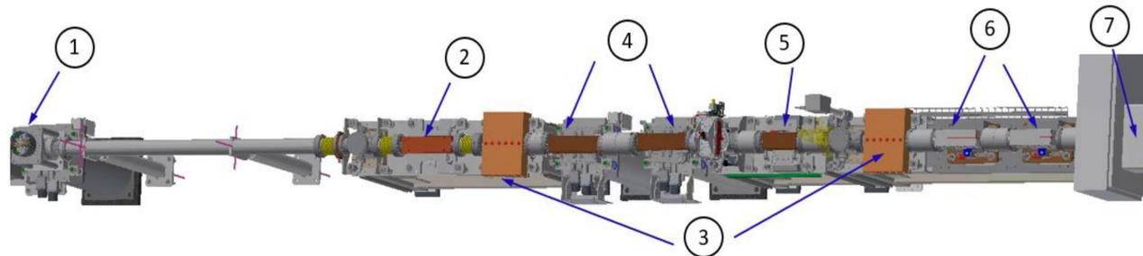
A typical NSLS-II ID front end; (1) XBPM, (2) fixed aperture mask (FM), (3) lead collimators (LCO), XY slits, (5) photon shutter (PS), (6) safety shutters (SS), and (7) ratchet wall collimator (RCO).
