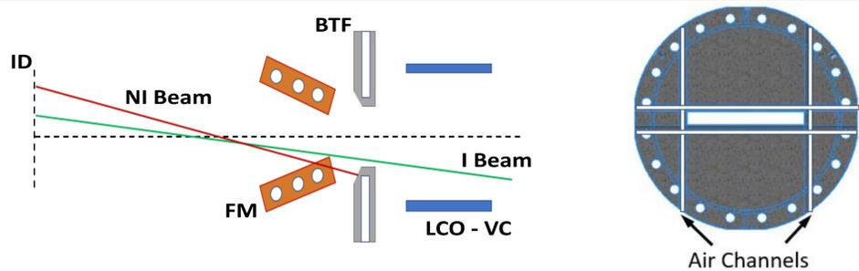
Burn-through flanges are used at NSLS-II to ensure that lead-collimator vacuum chambers are protected for large e-beam deviations.
