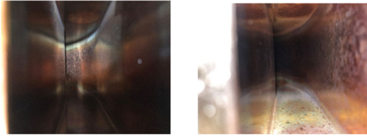
Figure 8: Stain at the WG bend/ bottom.
