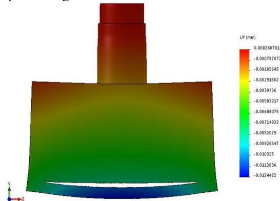
Figure 5: Deformation distribution diagram of the cooling seat in the vertical direction with a heat load of 62.89 W.
