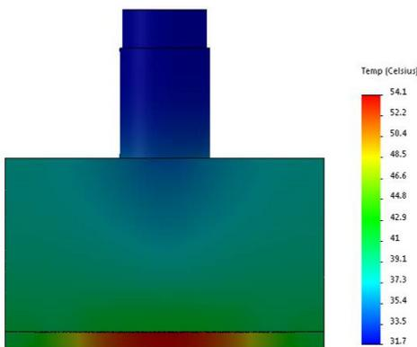
Figure 3: Temperature distribution diagram of the cooling seat under 62.89 W heat load.
