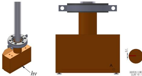
Figure 2: White beam position monitor measurement and beam light entrance size.
