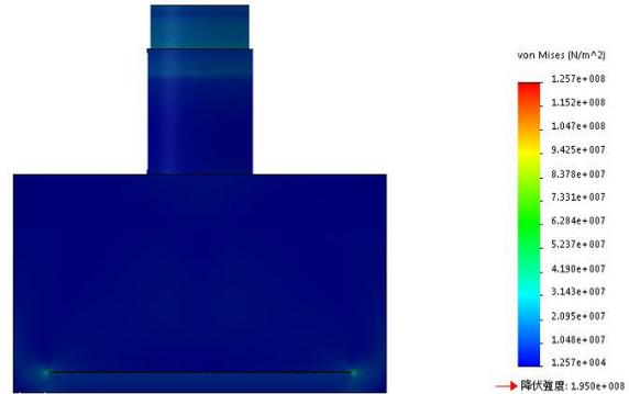
Figure 4: The cooling seat bears the stress distribution of 62.89 W thermal load.
