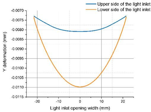
Figure 6: The data graph of the opening deformation of the cooling seat in the vertical direction under the heat load of 62.89 W.
