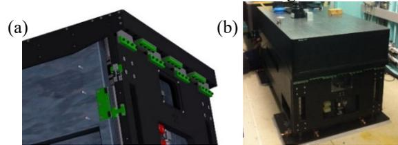
Figure 3: The KB Table at XFM beamline, Australian Synchrotron. a) Detailed view of the  $90^\circ$  Cross flexure hinge. b) picture of the KB table.
