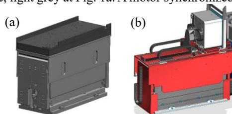
Figure 1: a) ALBA BL13 Diffractometer table. b) 3D model of the BL13 XALOC detector table.
