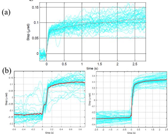
Figure 4: a) Resolution at 1 full step of the BL13 XALOC detector table. b) Resolution at 1 & 2 full steps (Figure b1 & b2) of the beam conditioning elements table for BL11 NCD-SWEET beamline.
