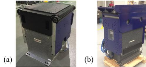
Figure 2: a) Sample Table for BL11 NCD-SWEET beamline with bearing articulated pitch. b) Beam conditioning elements table for BL11 NCD-SWEET beamline.
