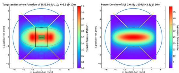
Figure 3: Example of the plots used to adjust the positions of the tungsten blades in the W-XBPMs. Left: tungsten response function plot. Right: power density plot.
