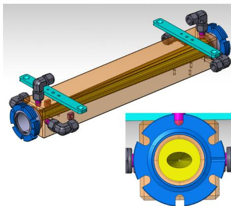
Figure 4: High power diaphragm. Insert bottom: cornerless entrance and exit window.
