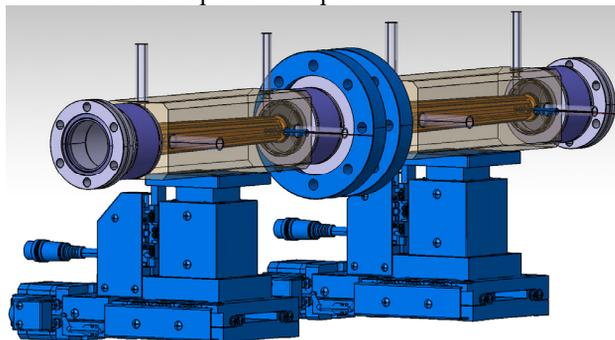
Figure 6: Draft of the new high power slits (design to be finished).
