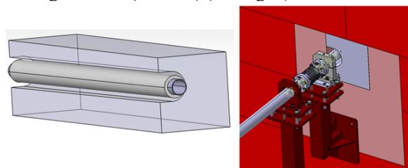
Figure 7: Tunnel wall break through. Left: casted mono block concrete filler with beam tube (surrounded with insulation for bake out). Right: Situation.
