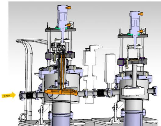
Figure 5: Cut through photon shutter (left) and beam stopper (right) with fast- and gate valve in between.
