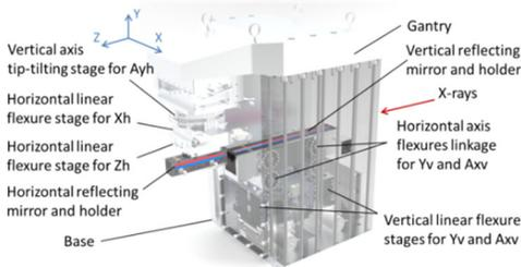
Figure 9: 3D model of the 4-ID-G ISN K-B mirrors with stage groups on a base with gantry structure in UHV.
