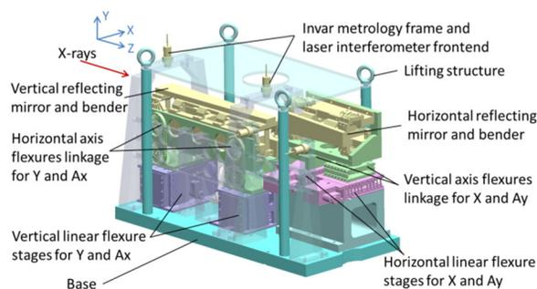
Figure 10: 3D model of the 9-ID-D nanofocusing K-B mirrors with flexure stage groups on the same UHV base.
