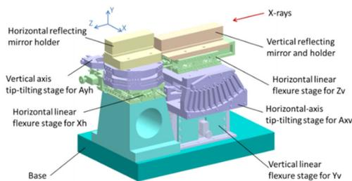
Figure 7: 3D model of the 7-ID-D nanofocusing K-B mirrors with flexure stage groups on same base in UHV.
