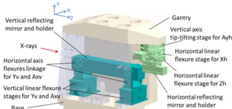
Figure 8: 3D model of the 19-ID-E ISN K-B mirrors with stage groups on a base with gantry structure in UHV.
