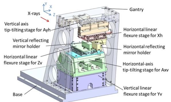
Figure 6: 3D model of the 32-ID nanofocusing K-B mirrors with separate flexure stage groups on a base with gantry structure.
