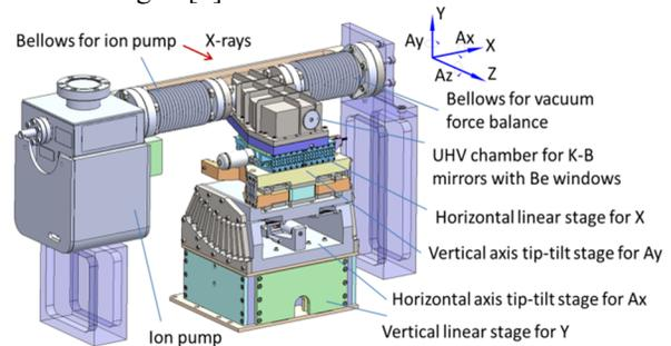
Figure 5: 3D model of the 34-ID-E Mini-UHV-Chamber with multidimensional flexure stage system.
