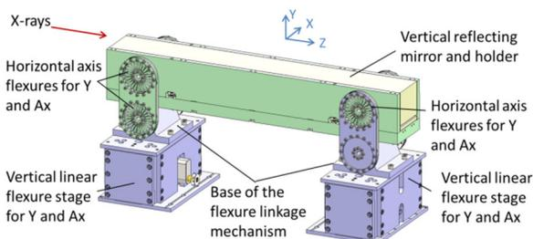
Figure 4: 3D model of the APS UHV-compatible flexures linkage mechanism for a 400-mm-long vertical reflecting mirror alignment apparatus.
