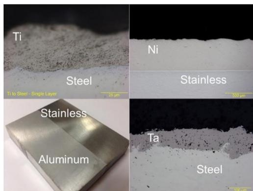
Figure 2: Example UAM dissimilar metal interfaces showing (a) titanium and steel (b) nickel and stainless steel (c) aluminum and stainless steel (d) tantalum and steel [4].
