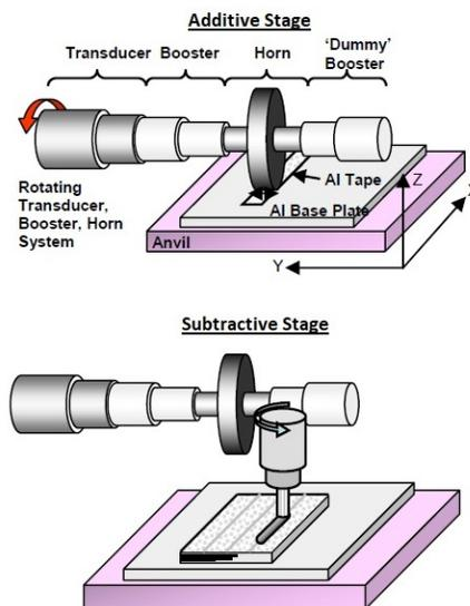
Figure 1: UAM process schematic showing additive and subtractive stages [1].
