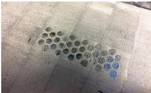
Figure 5:  $\text{Eu}_2\text{O}_3$  and Ta neutron absorbers embedded in a control panel used in a high-flux isotope reactor at ORNL [4,7].
