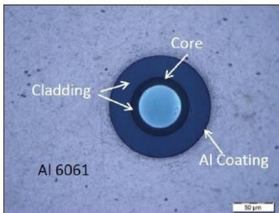
Figure 4: Metallized fiber optic cable embedded in aluminum 6061 fatigue specimen [6].
