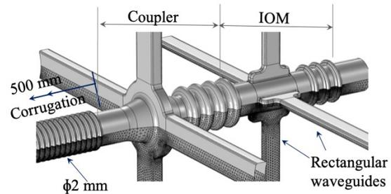
Figure 1: The corrugated waveguide and fundamental coupler followed by the IOM.
