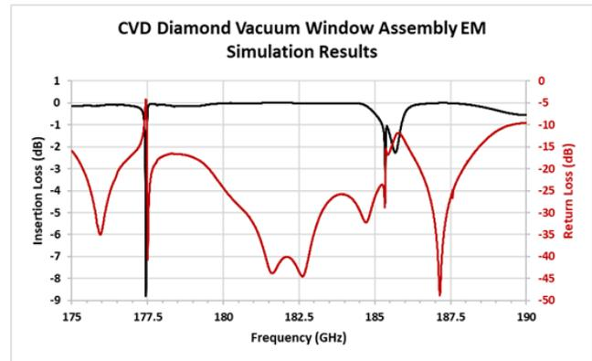
Figure 3: Electromagnetic simulation results from CST Microwave Studio of the entire vacuum window assembly, as shown in Fig. 2.
