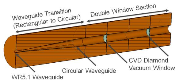
Figure 2: The entire window structure is shown. On the left is the rectangular-to-circular transition. In the center is the diamond window section, with the two windows shown.
