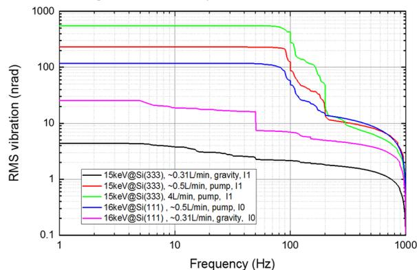
Figure 9: Integrated RMS displacement.
