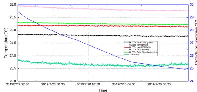
Figure 7: Temperature recordings during long-term stability test.
