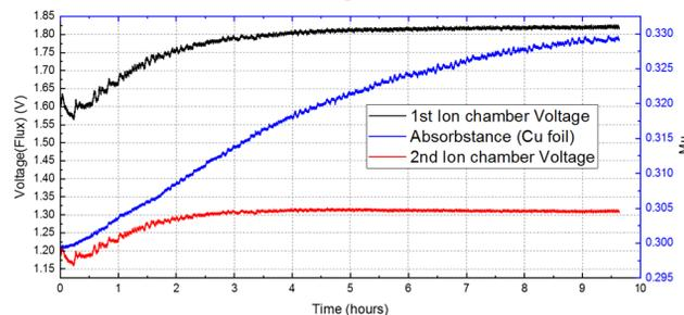
Figure 6: Cu K edge flux and absorption ratio for 9 hours.
