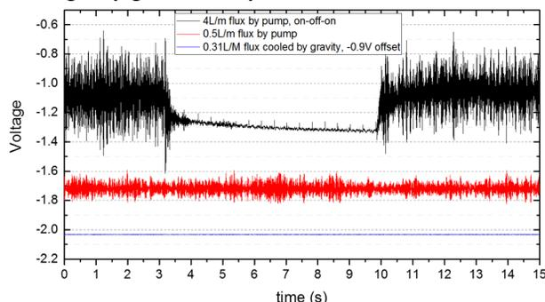
Figure 8: Ion chamber readings under different conditions.
