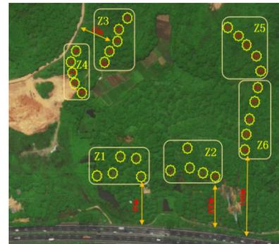
Figure 1: Distribution points of vibration measurement.
