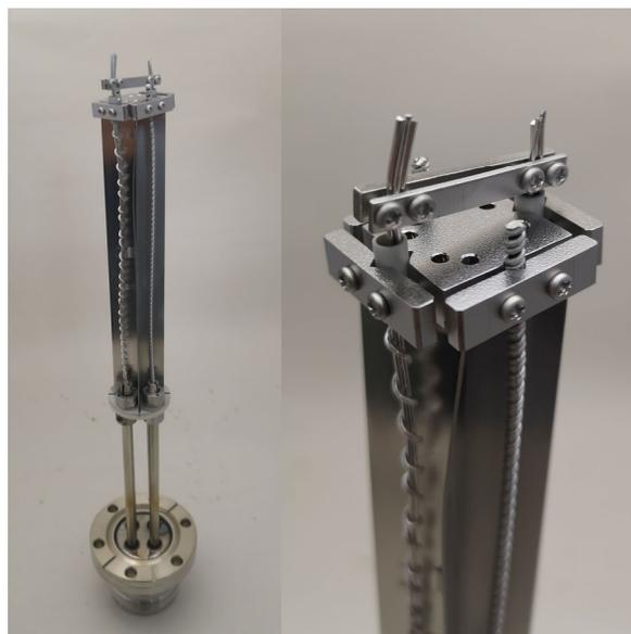
Figure 4: The Pd and Ti evaporator.
