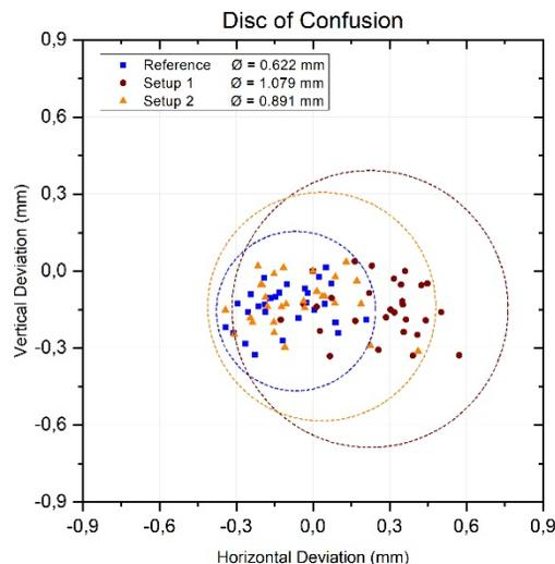
Figure 4: Disc of confusion of the acceptance test. It represents the minimum circumscribed circle for each data set and considers the setup estimated uncertainty.
