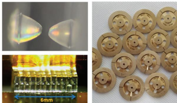
Figure 2: Top left: Side view of a double-sided lens. Bottom left: ultra-compact CRL made of diamond plate stack. Right: diamond lenses packaged in an aluminum-bronze holder.
