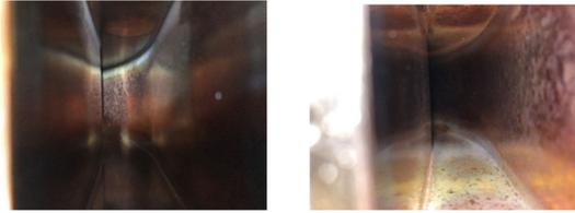
Figure 8: Stain at the WG bend/ bottom.
