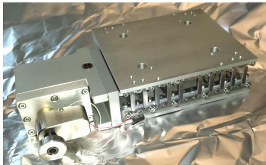
Figure 3: Photograph of the APS T8-48v04 UHV-compatible horizontal flexure stage.
