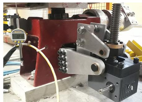
Figure 6: Prototype lever inserted in the magnet jack.
