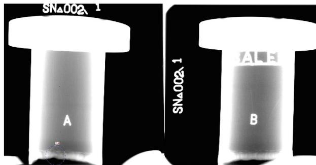
Figure 2: X-ray inspection of welds in the 2nd article, meeting Class A standard.
