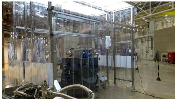
Figure 3: CAT M2 granite bench and UHV chamber inside a portable cleanroom laminar flow ready for the installation procedure.
