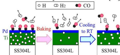
Figure 1: Schematic showing the activation and pumping mechanisms of oxygen-free Pd/Ti deposited on stainless-steel SS304L. Reproduced from Ref. [18].
