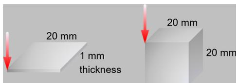
Figure 4: left: CVD diamond model, right: B<sub>4</sub>C
