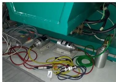
Figure 12: Velocimeters implementation on slab.
