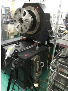
Figure 9: Horizontal direct drive spindle.
