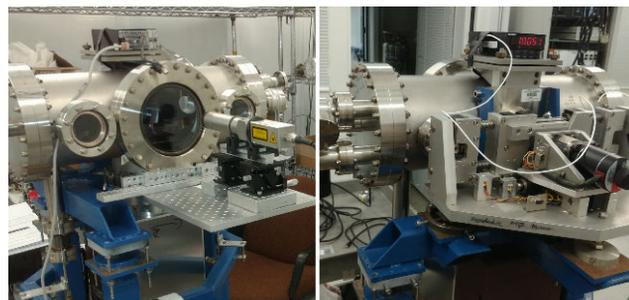
Figure 3: *In situ* autocollimator measurement of former SRC mirror prior to refurbishment for use as XTIP.
