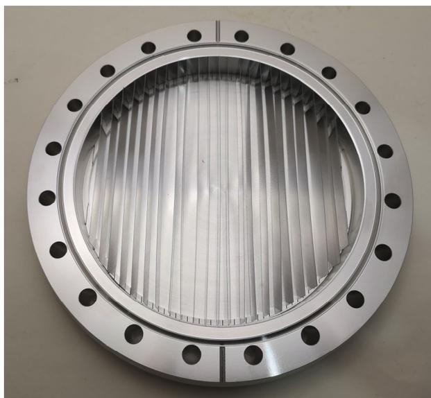
Figure 2: The vacuum vessel for the zero-length CF fin-type NEG pump before oxygen-free Pd/Ti deposition.
