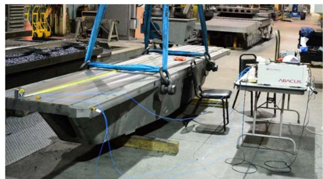
Figure 5: FODO prototype undergoing free BC EMA.
