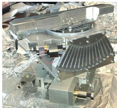
Figure 6: A photograph of the pilot nanositioning stages for CBXFEL diamond crystal manipulation.
