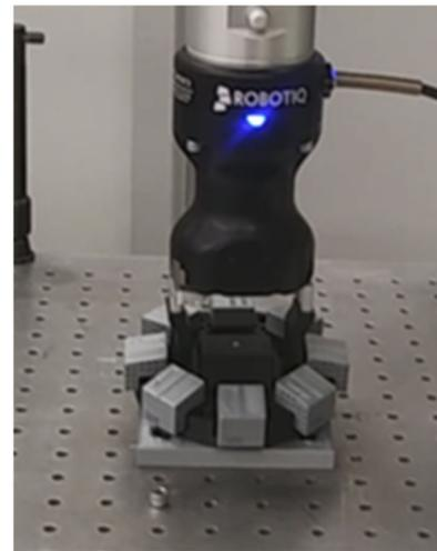
Figure 4: Sample wheel with Robot Gripper interacting 8-ID Lab test area.
