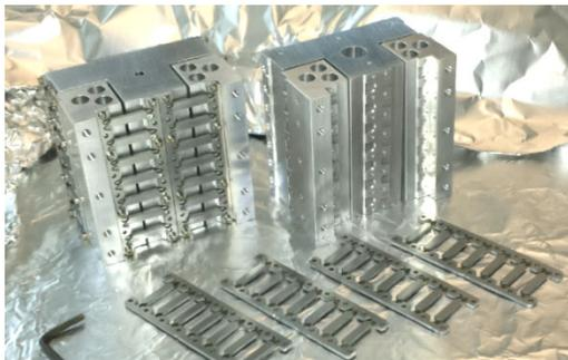
Figure 2: Photograph of the APS T8-49v02 vertical flexure stage weak-link guiding mechanisms.
