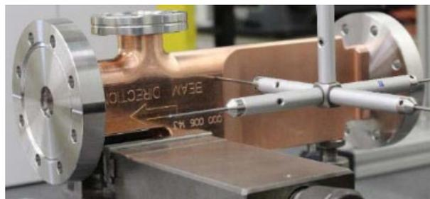
Figure 6: DS VC undergoing inspection.
