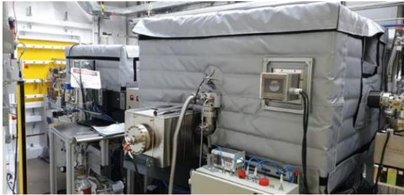
Figure 5: Setup of the "baking tent" used at the beamline, developed to avoid high temperatures outside the tent.
