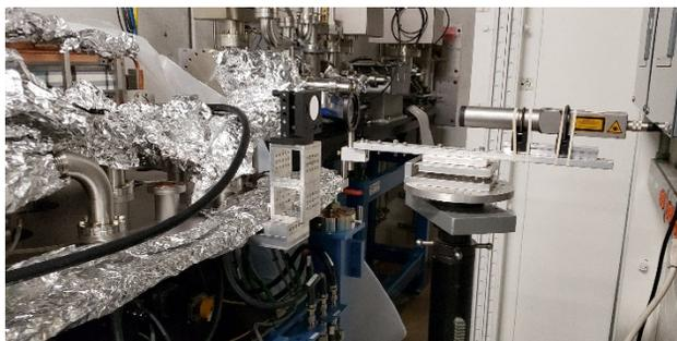
Figure 1: Autocollimator was aligned to us/in mirror at 2-ID prior to addition of reference mirror.
