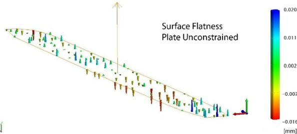
Figure 2: Measured flatness of DLMA girder, unconstrained and prior to mounting magnets.
