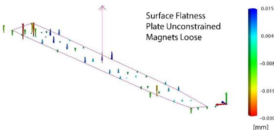
Figure 3: Measured flatness of DLMA girder, unconstrained and post mounting magnets.
