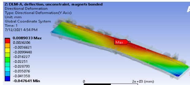
Figure 4: FEA simulated flatness of DLMA girder, unconstrained and post mounting magnets.
