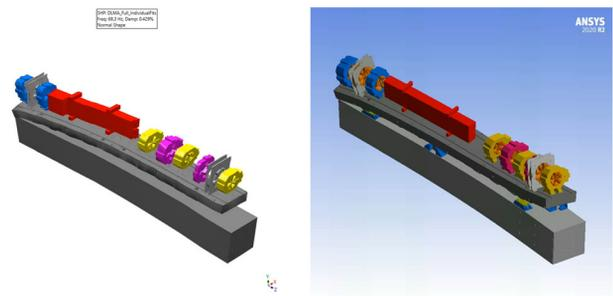
Figure 7: EMA (left) first mode shape at 68 Hz and FEA (right) first mode shape at 74 Hz.
