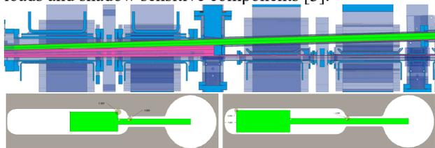
Figure 6: Top cross-sectional view of the ray trace through several chambers (top, beam direction from left to right), upstream (L) and downstream (R) cross-sectional view of the beam envelope (in green) within the keyhole chambers.
