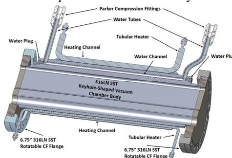
Figure 9: Top cross-sectional view of a SST keyhole chamber.
