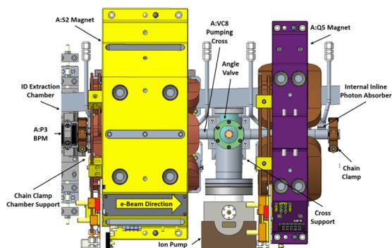
Figure 4: Top view of an aluminum pumping cross within a sextupole (left) and quadrupole (right) magnet.
