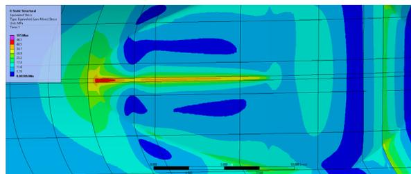
Figure 12: Von-Mises stress results on the inline photon absorber (maximum stress 46.3 MPa).
