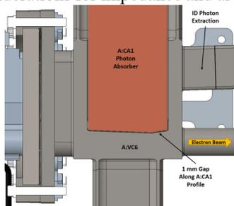
Figure 7: Top cross-sectional view of the discrete photon crotch absorber within the A:VC6 cross body.
