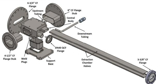
Figure 10: Exploded view of the A:VC6 cross design.
