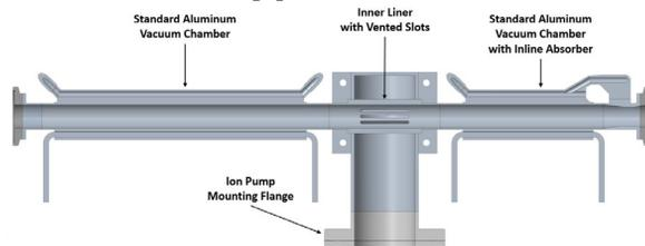
Figure 8: Top cross-sectional view of a NEG-coated Al cross.
