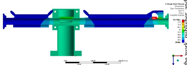
Figure 11: Top cross-sectional view of temperature results of the pumping cross FEA (max temperature of 83.7°C).
