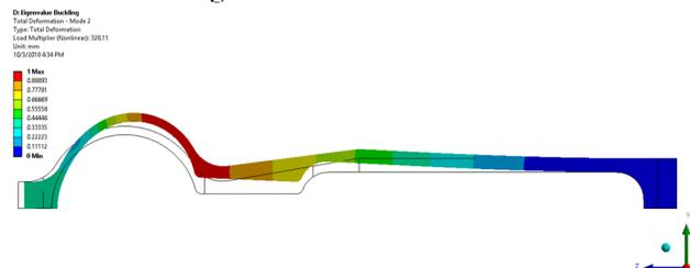
Figure 13: Critical load found to be 328 atm from buckling FEA for the keyhole chambers.
