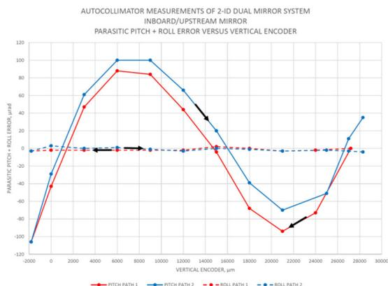
Figure 2: *In situ* autocollimator measurement of parasitic pitch and roll of the 2-ID us/in mirror.
