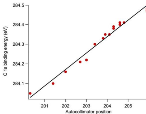
Figure 5: *In situ* autocollimator data from 4-ID-C SGM correlated with XPS measurements.
