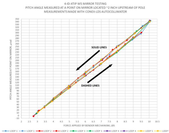
Figure 4: *In situ* autocollimator data of former SRC mirror prior to refurbishment for use at XTIP.
