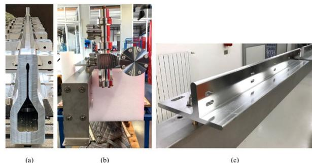
Figure 1: IDVC extrusion profiles throughout the fabrication process, 1a shows the VC, 1b shows a side view of the SB profile, and 1c shows the modified l-bracket profile.
