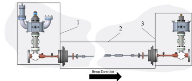
Figure 4: SCU VC assemblies, (1) US out-of-cryo VC, (2) in-cryo VC, and (3) DS out-of-cryo VC.
