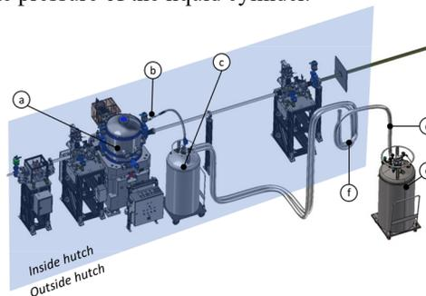
Figure 1: Third optical hutch of the CARNAÚBA beamline, highlighting the liquid nitrogen supply system of the 4CM, which comprises the vacuum chamber (a), the cryostat (b), the primary (c) and secondary (e) LN2 cylinders, the transfer line (d) and the exhaust line (f).
