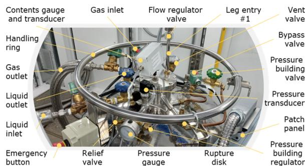
Figure 2: Top of primary LN2 cylinder and description of the connected elements.
