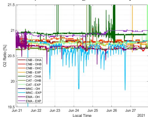
Figure 5: O2 ratio in several optical (OH) and experimental (EXP) hutches of CARNAÚBA, CATERETÊ, MANACÁ and EMA beamlines.
