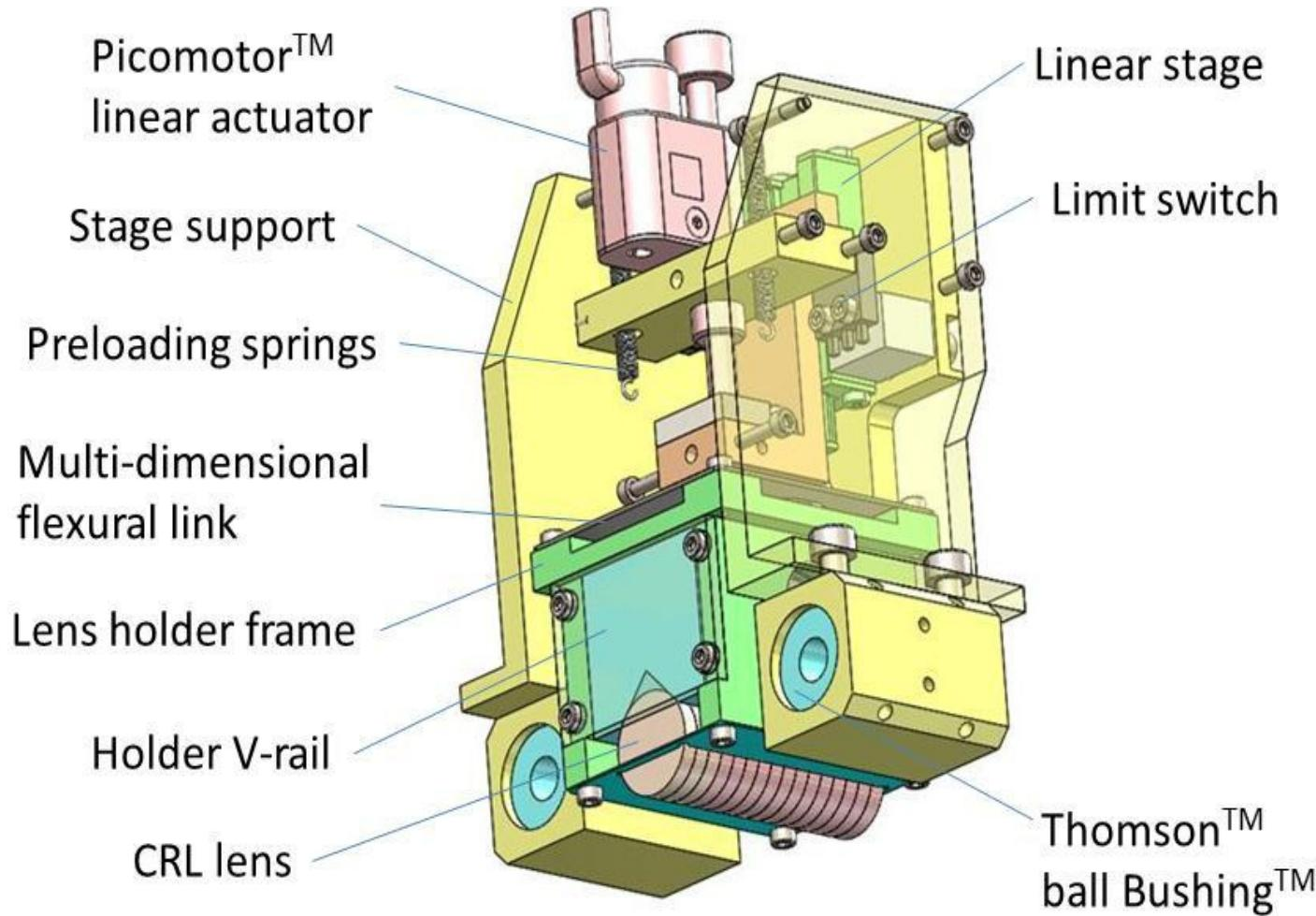
To manipulate CRL lens stack with longer total length, a compact manipulator APS Y9-5102 for 32-mm CRL lens stack was designed using commercial piezo-driven linear actuator, such as Picomotor™ 8353, as a lens manipulating driver with maximum axial driving force of 13 N.
