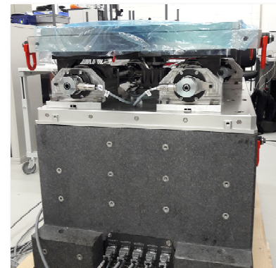
Chamber is supported by movers with eccentric cam-shaft drivers and on a granite block
