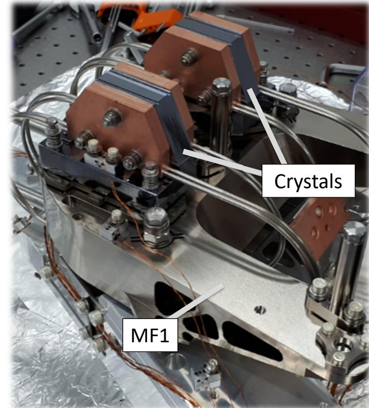
\*Manifold assembly mounted to brazing tooling.
