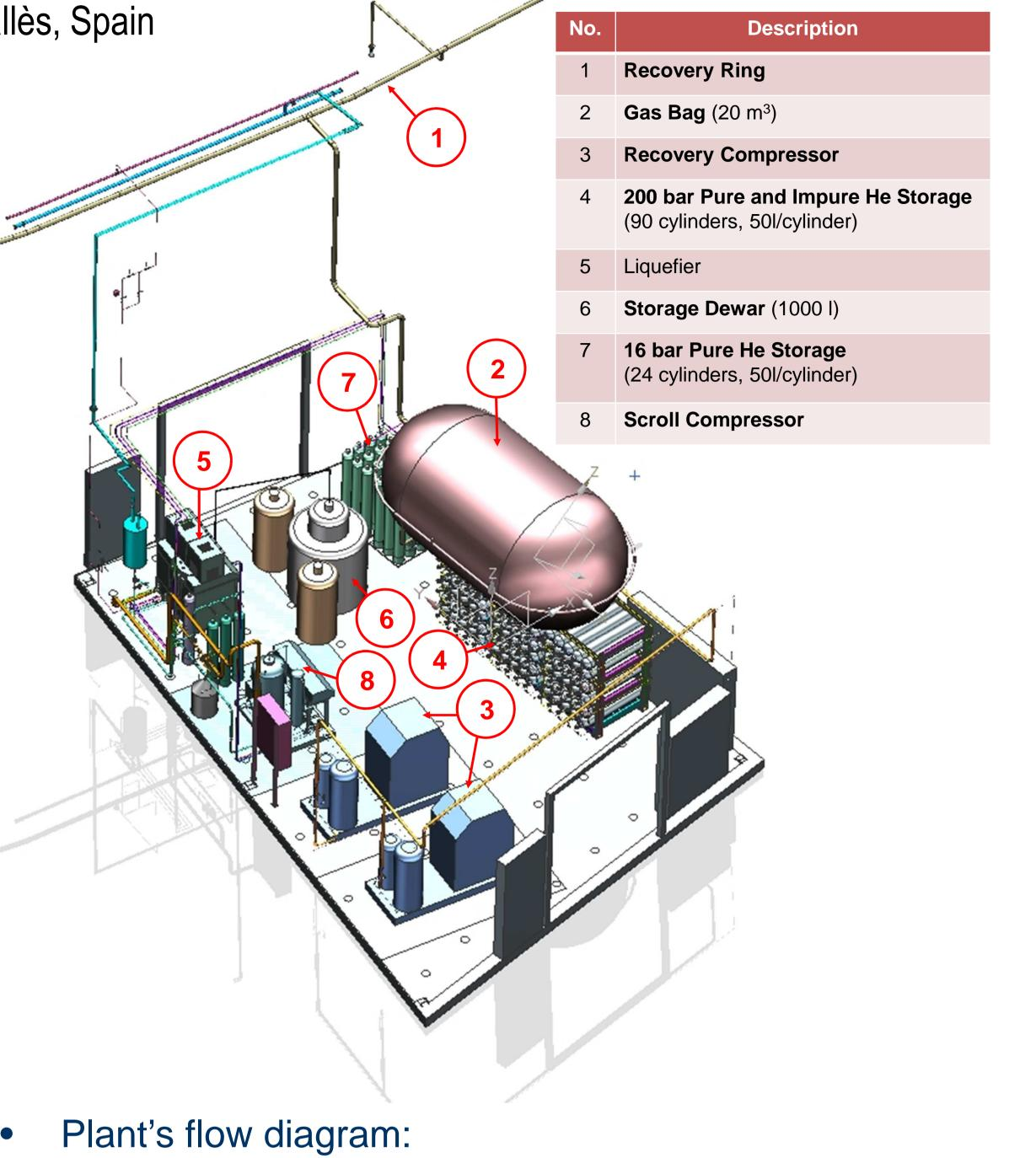
recycling up to 24960 litres of LHe per year, which is an 80% of the helium consumed at ALBA, by making the gaseous helium undergo through 3 main stages: recovery, purification and liquefaction.
