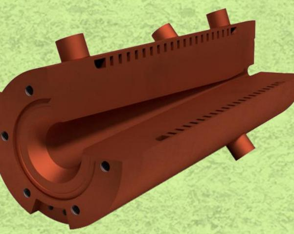
Three-quarters view of a component. It is possible to notice the water chamber and the flange machined on the CuCrZr bulk.
